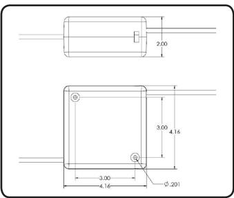
Reel Material ABS plastic Retraction Length 6 ft (1.8 m) Static Length 3 ft (0.91 m)
